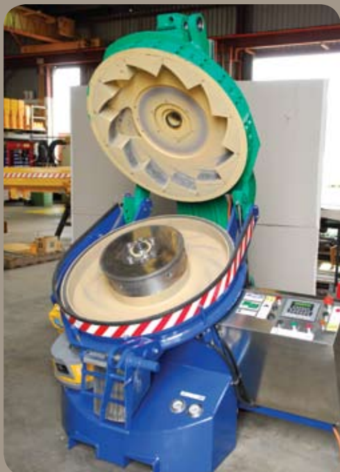
The inside of a commercial JK Rotary Breakage Tester characterisation device. Image © JKMRRC.
